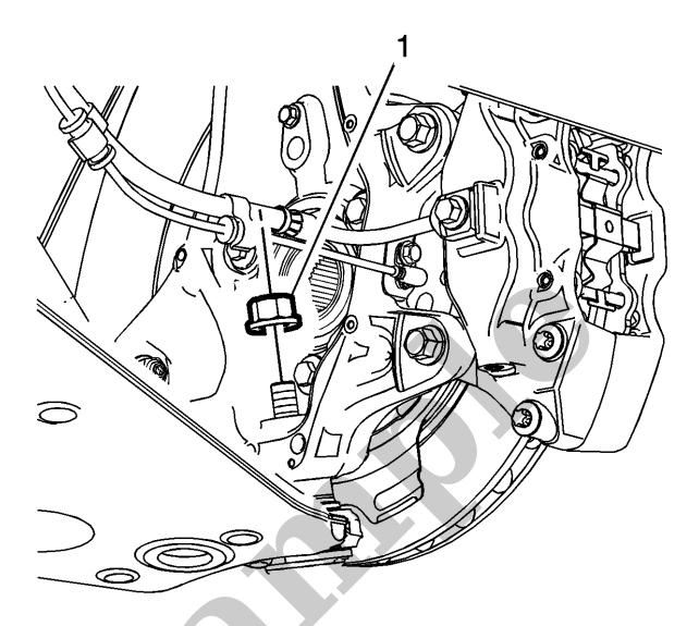
Remove and DISCARD the rear axle lower control arm ball joint nut(1).
