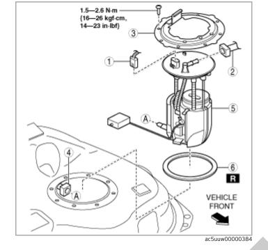
1 Fuel pump unit connector Quick release connector 2 (See QUICK RELEASE CONNECTOR (FUEL SYSTEM) REMOVAL/INSTALLATION [SKYACTIV-G 2.5 (WITHOUT CYLINDER DEACTIVATION)].) 3 Set plate Quick release connector 4 (See QUICK RELEASE CONNECTOR (FUEL SYSTEM) REMOVAL/INSTALLATION [SKYACTIV-G 2.5 (WITHOUT CYLINDER DEACTIVATION)].) 5 Fuel pump unit 6 Packing
