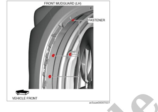
7.Partially peel back the front mud guard (LH) to a position allowing removal of the relay box (LH).
