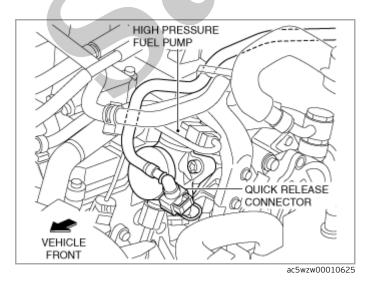
4.Connect a long hose to the disconnected quick release connector and drain the fuel into a container used for collecting gasoline.
