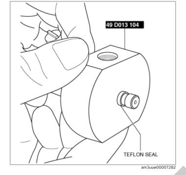
9. Hold the SST at the position shown in the figure and correctly position the teflon seal for more than 30 sec.
