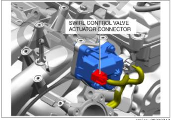
4. Connect the swirl control valve position sensor connector shown in the figure.
