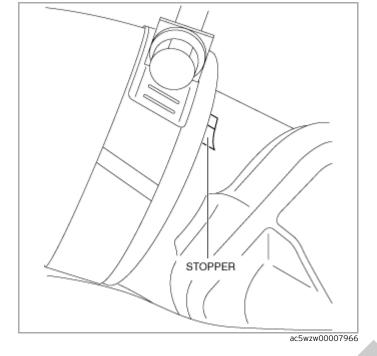
5.Re-position the temporarily installed hose clamp to the position 5–7 mm (0.20–0.27 in) from the charge air cooler outlet pipe stopper.
