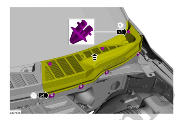
3. Disconnect the windshield washer tube and remove the cowl panel grille.
