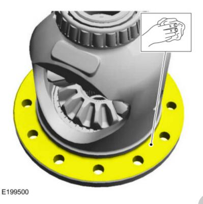
5. Using the special tools, remove the LH (left-hand) differential bearing.
