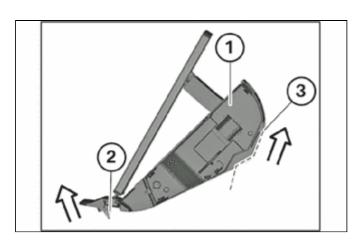
(e) Slide the accelerator pedal sensor assembly (1) out of the holder (3) in the direction of arrow (diagonally upwards).
