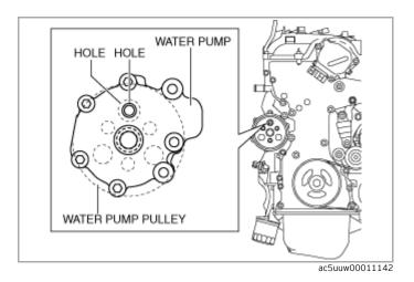
2.Insert an appropriate bolt (length 70 mm {2.8 in}) into the water pump hole shown in the figure and lock the water pump pulley against rotation.
