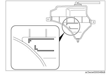
• If the engine coolant level is below the L mark, add engine coolant.
