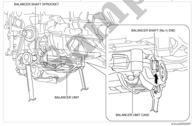
(2) Tighten the balancer shaft sprocket installation bolt.
