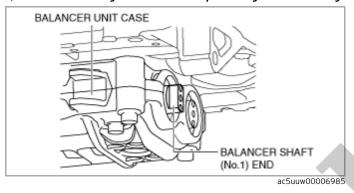
(1)Lock the balancer shaft (No.1) against rotation as shown in the figure.
