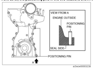
1.If the engine front cover is newly replaced, tap the positioning pins in the two locations to the seal surface side.
