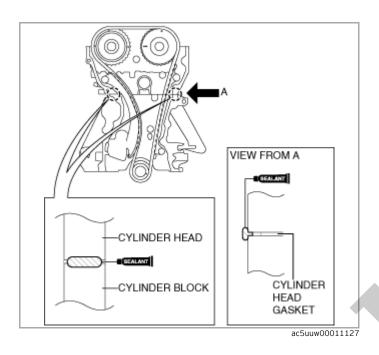
7.Install the engine front cover to the engine.
