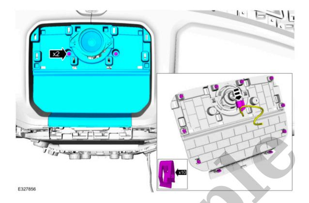
32. Release the clips and remove the LH (left-hand) instrument center trim panel.
