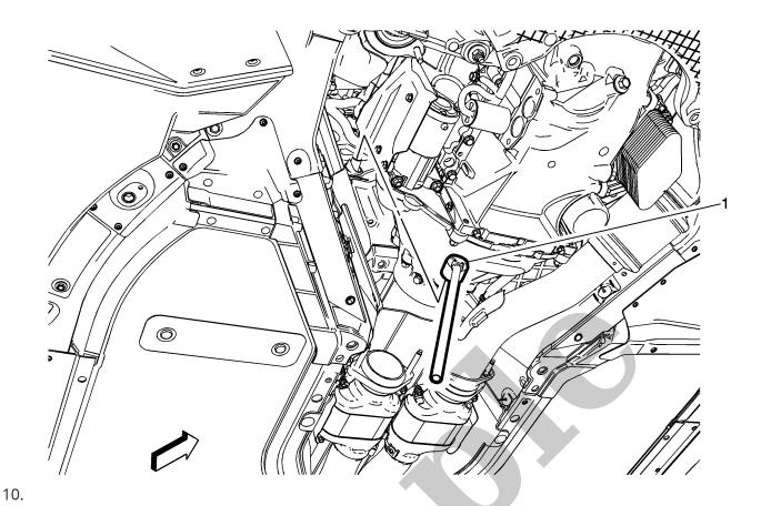
Remove the air conditioning evaporator and blower module drain tube (1). Air Conditioning Evaporator and Blower Module Drain Tube Replacement
