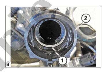
(i) Connect No. 6 radiator hose on No. 2 radiator assembly for low-temperature cooling system and lock.
