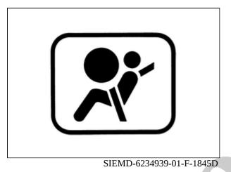
• For operation check purposes, air bag warning lamp turns ON for 7 seconds after power switch is turned ON. During this period of time, air bag diagnosis sensor unit performs system diagnosis.
