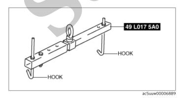
4.To ensure the safety of the work (control engine and transaxle sway), set a hoist as shown in the figure.
