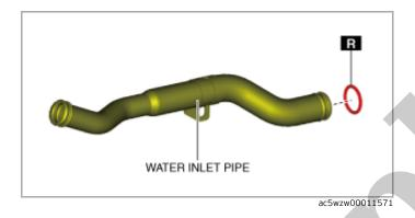
3.Insert the water inlet pipe into the water pump so that the marked position is aligned with the projection position.
