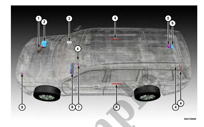
The Remote Starting system can consist of the following components:
