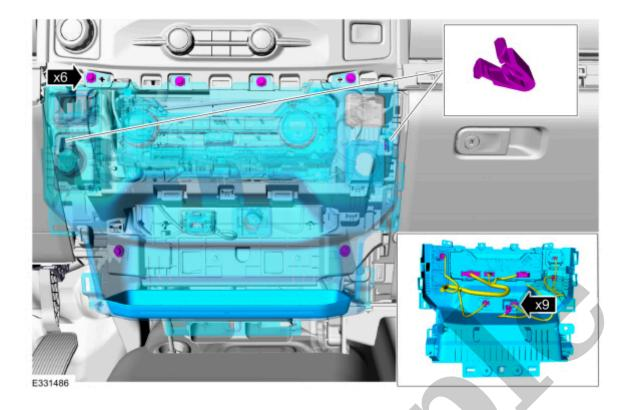
62. Disconnect the FM2/diversity amplifier to audio unit antenna cable connector from the FM2/diversity amplifier.
