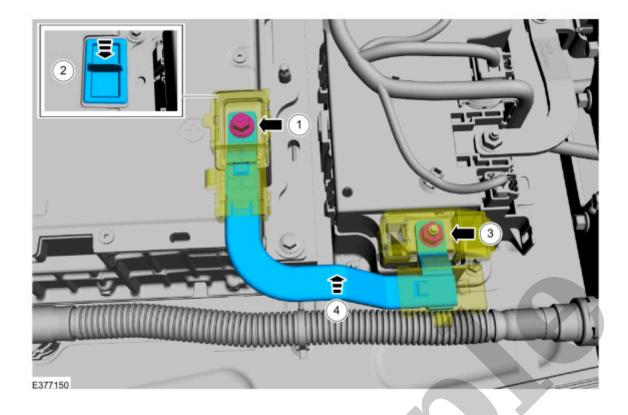
8. Detach the retainers, disconnect the electrical connectors and position the wire harness aside.
