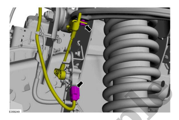
4. Remove and discard the upper arm bolts and nuts and remove the upper arm.
