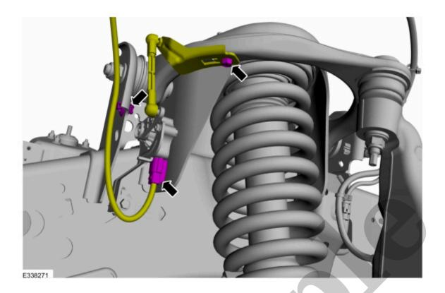
6. Calibrate the suspension system. Connect the scan tool and carry out the Ride Height Calibration routine. Follow the scan tool directions.
