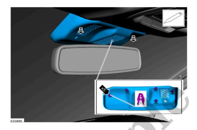
7. Disconnect the headliner wiring harness electrical connectors.
