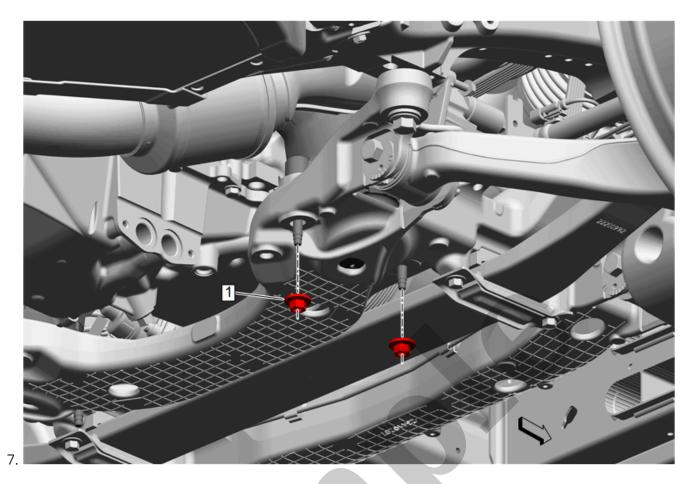
Engine Mount Nut(1)-Right Side »Install[2x]— Engine Mount Replacement - Right Side
