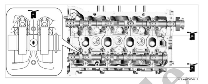
5. Apply SAE 90 gear oil or equivalent, or engine oil to the thrust surface of the front camshaft cap.
