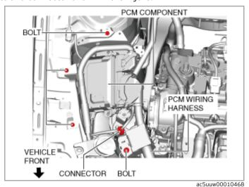
(2)Move the PCM component in the direction of the arrow shown in the figure and set it aside with the PCM connectors connected.
