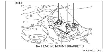
2.Tighten the No.1 engine mount bracket B installation bolts in the order shown in the figure.
