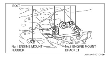
2.Tighten the No.1 engine mount bracket installation bolts in the order shown in the figure.
