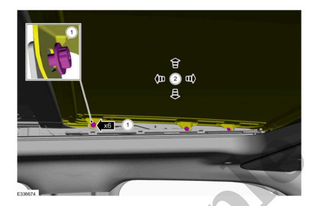
6. If any adjustment was made on the roof opening panel fixed glass roof opening panel fixed glass panel, initialize the roof opening panel.
