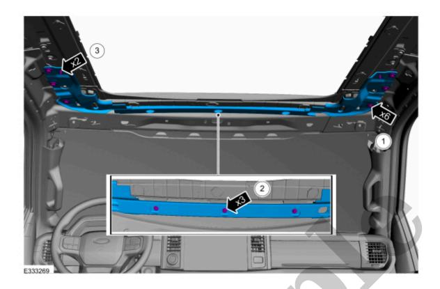
9. Disconnect the rear drain tubes and the roof opening panel motor electrical connectors.
