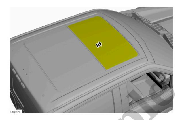
2. Measure the rear and sides of the rear fixed glass to roof clearances as shown.
