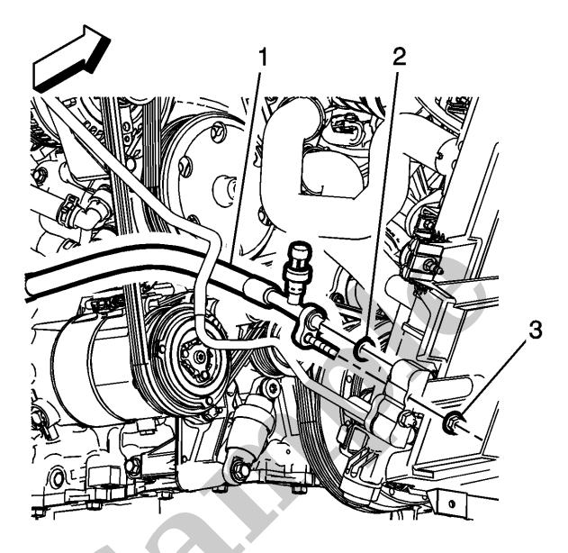
Install the air conditioning compressor and condenser hose (1) to the condenser. Air Conditioning Compressor and Condenser Hose Replacement
