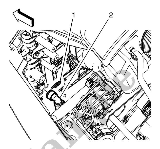
Remove the engine oil cooler coolant outlet hose (2) from the radiator. Engine Oil Cooler Coolant Outlet Hose Replacement
