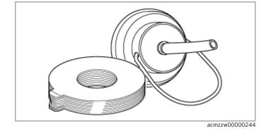
6.Insert the EVAP/low pressure vapor output hose nozzle into the gas cap single thread hose as shown in the figure.
