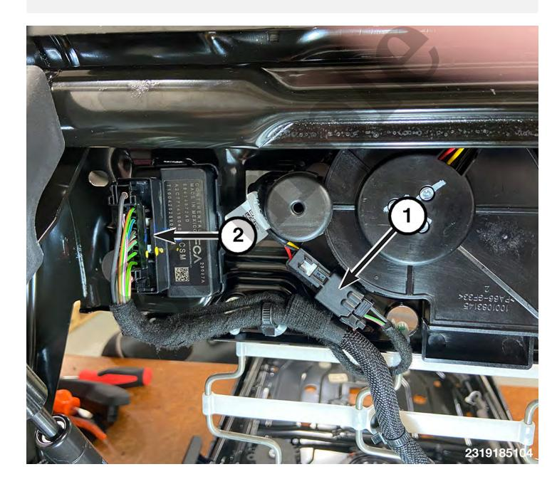
1 - Vent Fan Motor - Long Wheel Base
