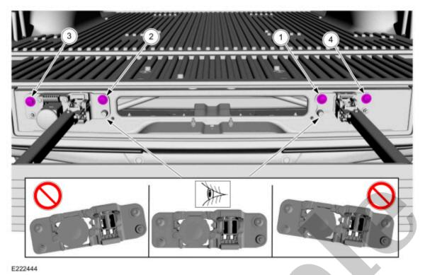
9. Cycle the tailgate step fully open and closed several times, ensuring the tailgate step fully latches in the closed position each cycle. If the tailgate step is still binding, repeat 2-8.
