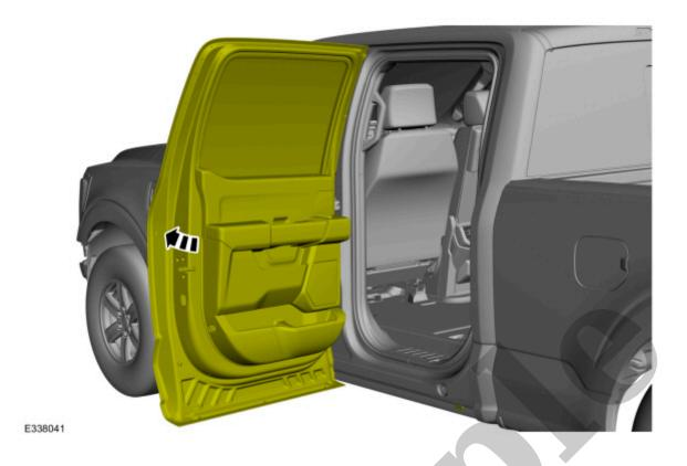
4. Loosen the bolts enough to permit movement of the door.
