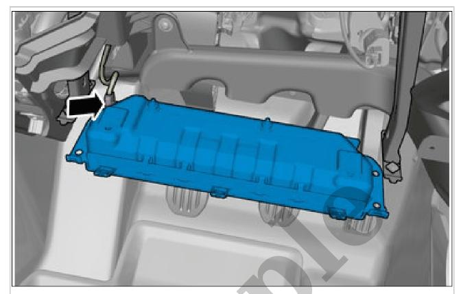
Disconnect the connector. Remove the marked part.
