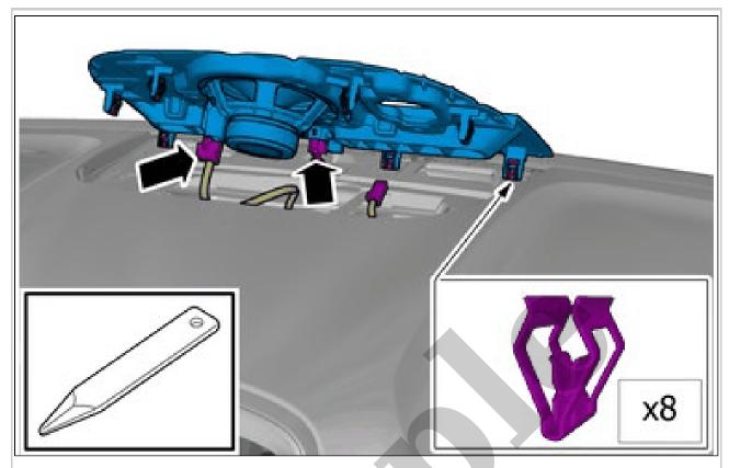
Remove the part carefully **Use:** Interior trim remover Disconnect the connectors. Remove the marked part.
