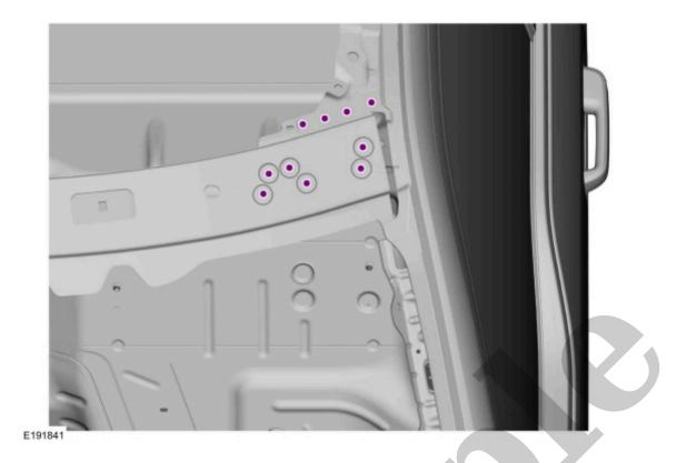
5. Break the adhesive bond and remove the roof front frame.
