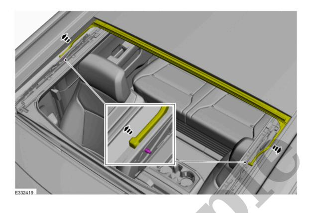
3. Pull the trough assembly towards the front of the vehicle and remove the trough assembly.
