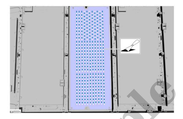
9. Remove the Thermal Interface Material (TIM) application template from the cold plate.
