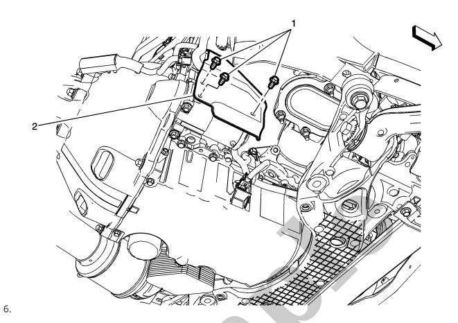
Remove the starter heat shield fasteners (1) and remove the starter heat shield (2) from the starter.
