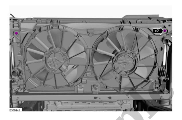
8. Lift the cooling fan motor and shroud upward and place wooden block to support it. Detach the pin-type retainers that secure the lower radiator shield to the cooling fan shroud.
