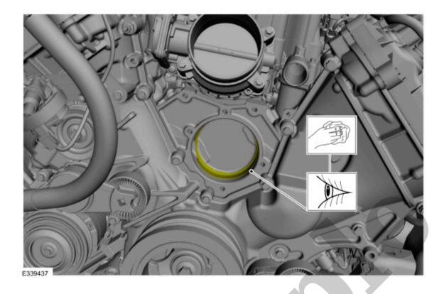
3. Install a new O-ring seal and lubricate it with clean engine coolant.
