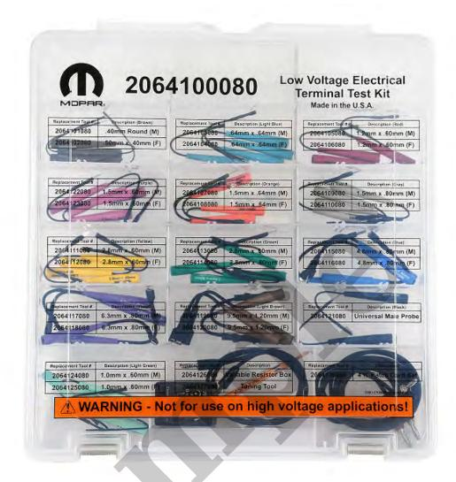
and insert the probing end (2) into the terminal being tested. Use the other end of the tool (1) to insert the meter probe. Use an ohmmeter to check the switch resistances as shown in the Remote Radio Switch Test chart; and then go to **Step 13**
