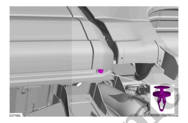
2. Using a non-marring trim tool, detach the retainers and remove the lower cab corner moulding.
