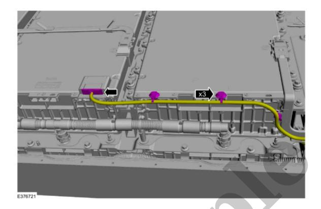
9. 1. Open the terminal cover and remove the bus bar bolt.
