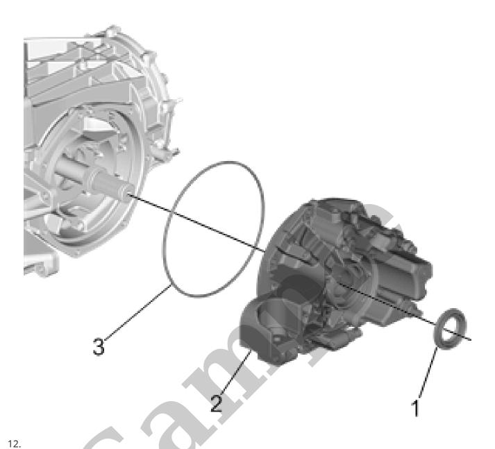
Remove the differential cover (2) from the differential.
