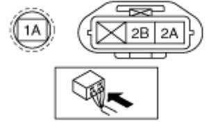
PCM WIRING HARNESS-SIDE CONNECTOR
