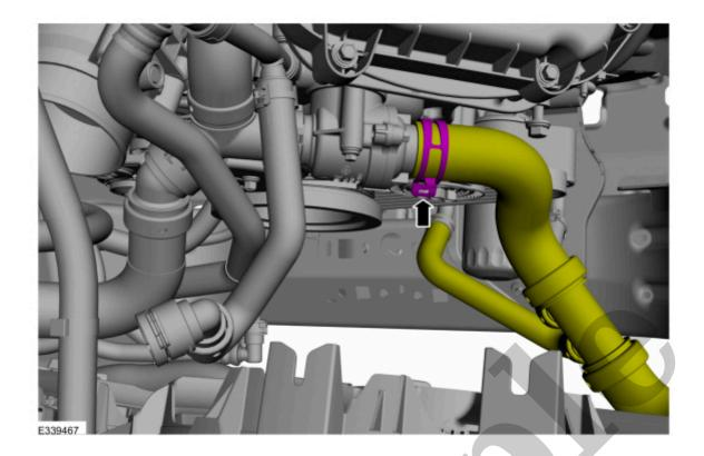
6. Pull the upper radiator hose T-connector spring clip up until the end of the clip is in the detent on the quick connect coupling and disconnect the upper radiator hose.
