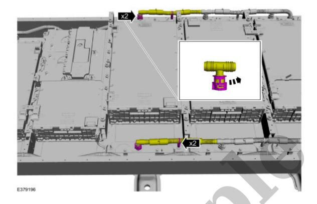
13. 1. Install the battery array lift adaptors.
