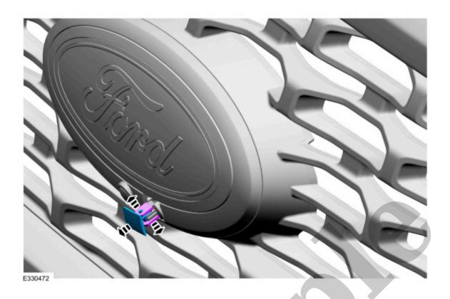
3. Remove the screws and the front camera washer and bracket as an assembly.
