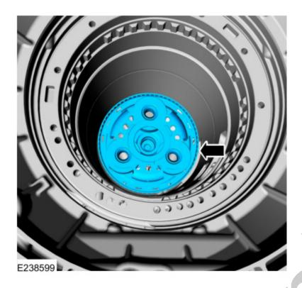
236. Remove the bolt and allow the park override lever to return to the normal operating position.
