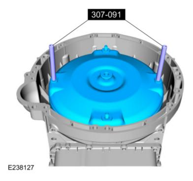
54. Install the special tool to hold the torque converter.
