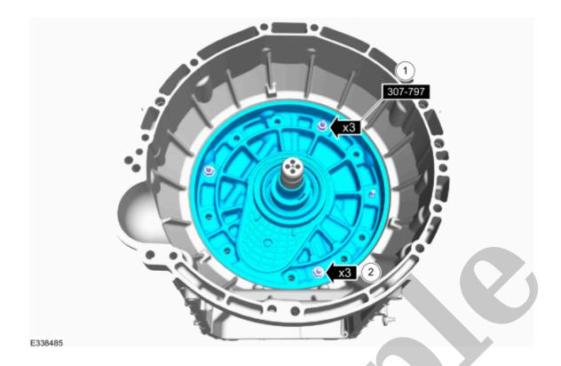
50. Install the new front support assembly bolt washers.
