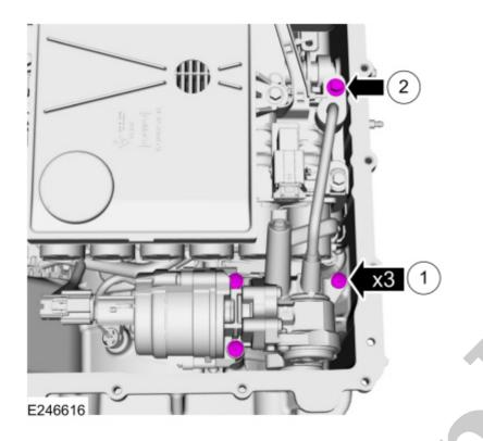
69. Connect the transmission fluid auxiliary pump electrical connector.
