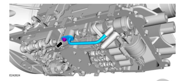
3. Remove the transmission fluid auxiliary pump tube seal.
