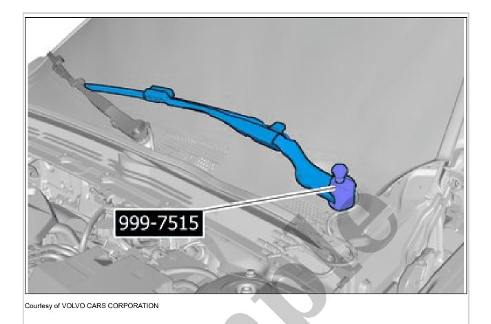
Special Tool: 999 7515 Puller Remove the marked part.
