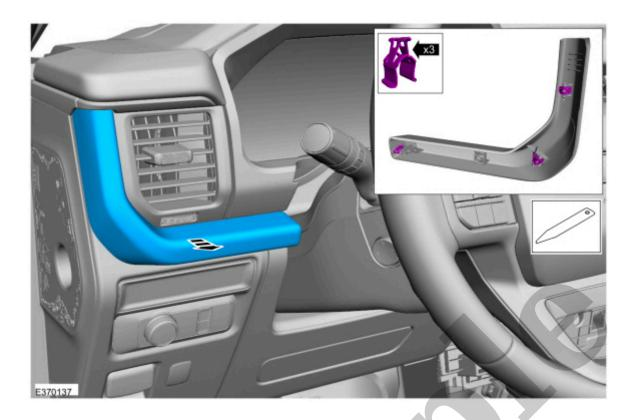
22. Release the retainers and remove the upper LH (left-hand) regsiter trim panel.
